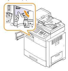
Pull up on the stacker lever and then close the stacker front cover.
